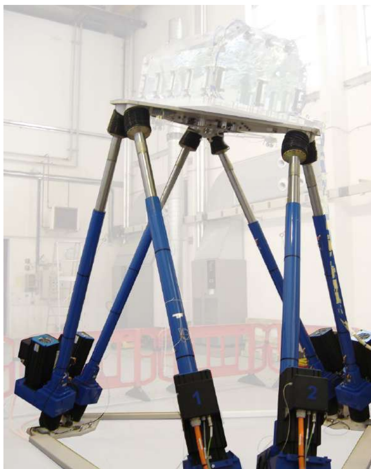
Hexapod AQUILON for sloshing tests.
