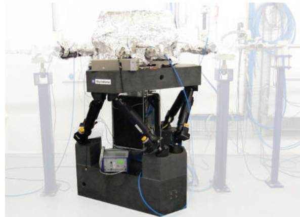
JORAN hexapod has been developed in collaboration with ESRF synchrotron to position mirrors with very high resolution.
