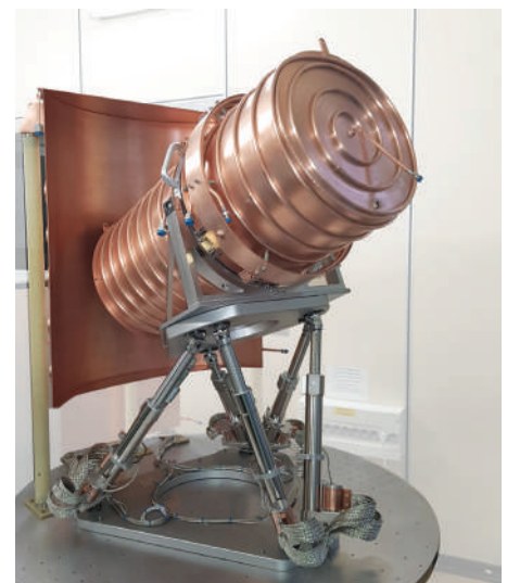
This HV ZONDA hexapod is used for the thermal vacuum tests and calibration of some of the cameras of PLATO mission at IAS.
