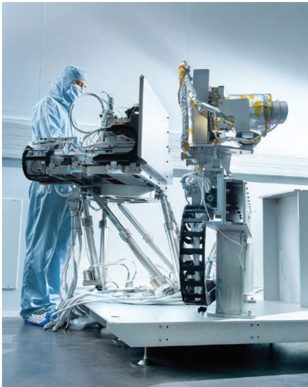
ISO5 clean room compatible hexapod to test space optical instruments for MTG (Meteosat Third Generation) satellites at BERTIN Technologies.
