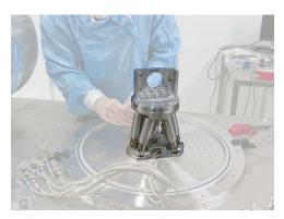
Two HV BORA hexapods are positioning the high reflectivity mirrors of a Fabry-Perot cavity in order to optimize their alignment and thereby the cavity finesse.
