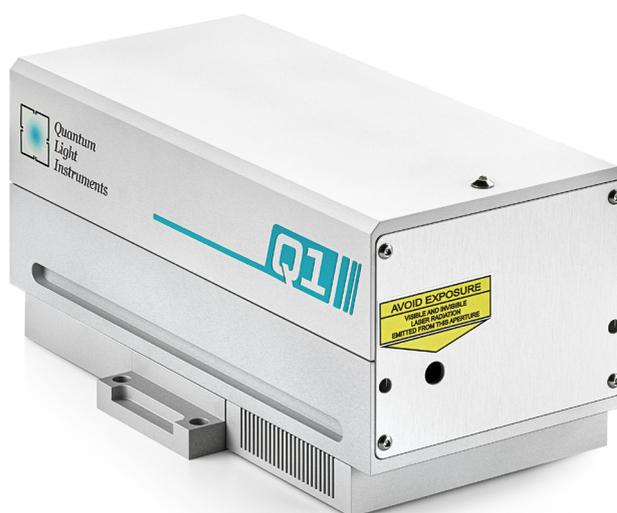
Q1 is compact, energy-efficient, diode pumped, air-cooled, Q-switched laser designed for wide range of applications that require high peak power pulses. Laser can produce up to 45 mJ at 10 Hz pulse repetition rate or up to 10 mJ at 50 Hz pulse repetition rate. Low divergence of laser beam allows efficient conversion to harmonic wavelengths using optional H1 series harmonic generator module.
